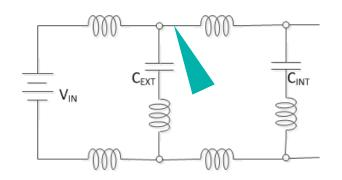
Partitioning C<sub>IN</sub> creates a higherorder Pi-network effect – 4<sup>th</sup> order roll-off.
